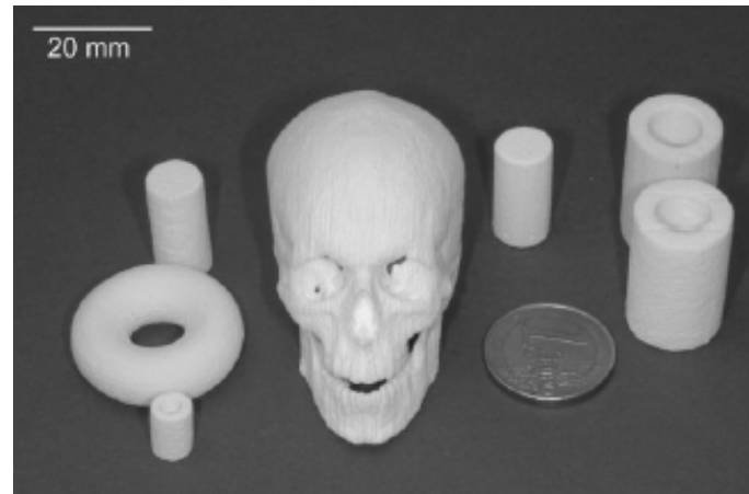
Tricalcium Phosphate (TCP) powder bound with phosphoric acid
